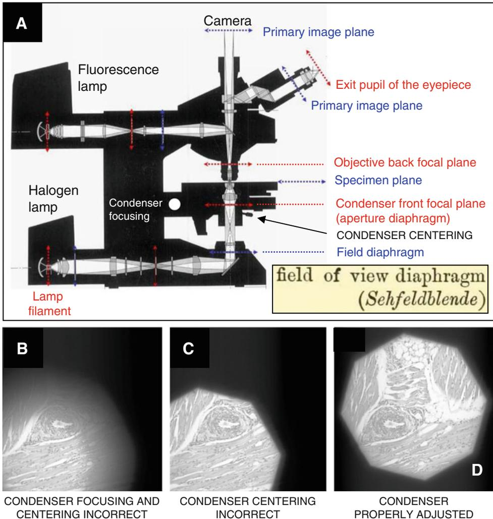
**Fig. 1** Optically conjugate planes of an upright microscope. **(A)** Imaging and aperture planes are marked in blue and red, respectively. Adapted from Ref. [39] by permission of © Elsevier. Note the original designation of the “field diaphragm” was “field-of-view diaphragm” (*Sehfeldblende* in German). The framed text is reproduced from Ref. [5]. **(B–D)** Field diaphragm as viewed through the eyepiece while centering the condenser (images by Dr. Lisa Cameron); see Appendix 2 for details
