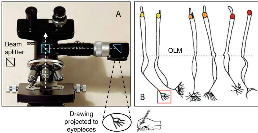
**Fig. 10** Camera lucida or drawing attachment. **(A)** Example of fitting to Wild M20-EB microscope. Adapted from Ref. [48] (© Ian Walker). **(B)** Camera lucida drawings of freshly isolated chick retina photoreceptor cells (cones) aligned by the outer limiting membrane (OLM). The color spots are oil droplets acting as color filters aiding color vision. Adapted from Ref. [49] (©López-López et al.)
