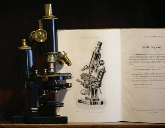
**FIGURE 8** An antique Koristka microscope, large model IIC with wide tube ideal for photomicrography. Appeared in a Koristka catalog published in 1908. From the Diatom Lab collection
