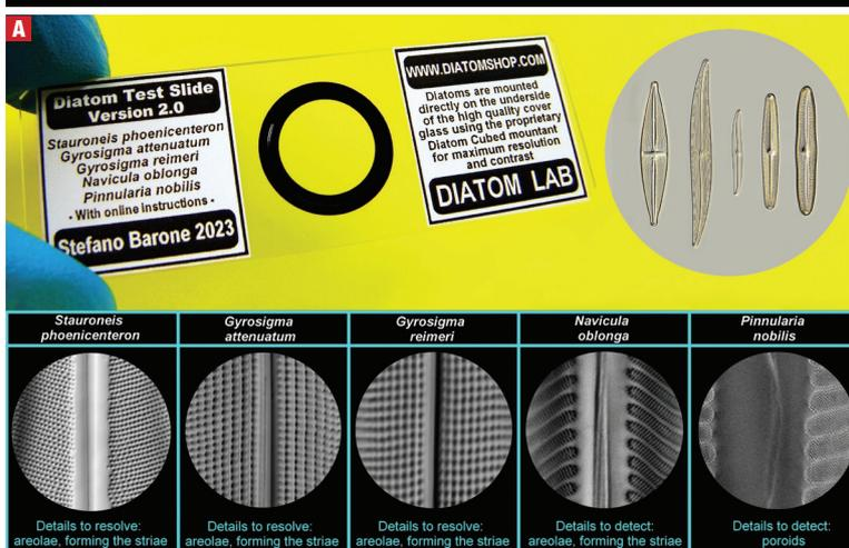
**FIGURE 2A**, top, The Diatom Test Slide Version 2.0 by Diatom Lab with its five selected, micromanipulated diatoms at low magnification and their resolved details;
