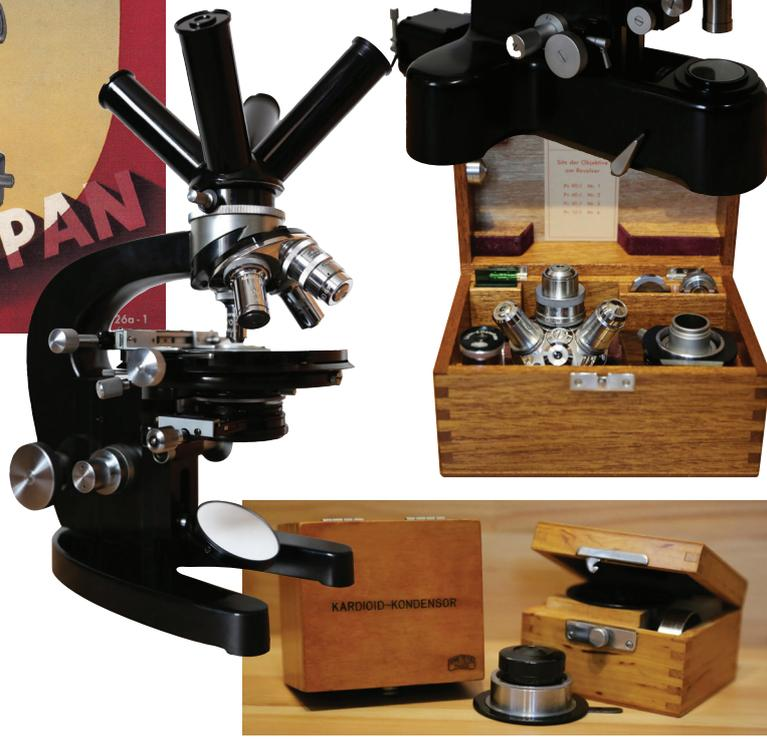
**FIGURE 7, above, A Zeiss Jena black enamel L Wd E microscope produced in 1941, equipped with the extremely rare Zeiss Jena ocular revolver. and, above right, two Zeiss Jena Siedentopf cardioid condensers for dark field illumination. From the Diatom Lab collection**
