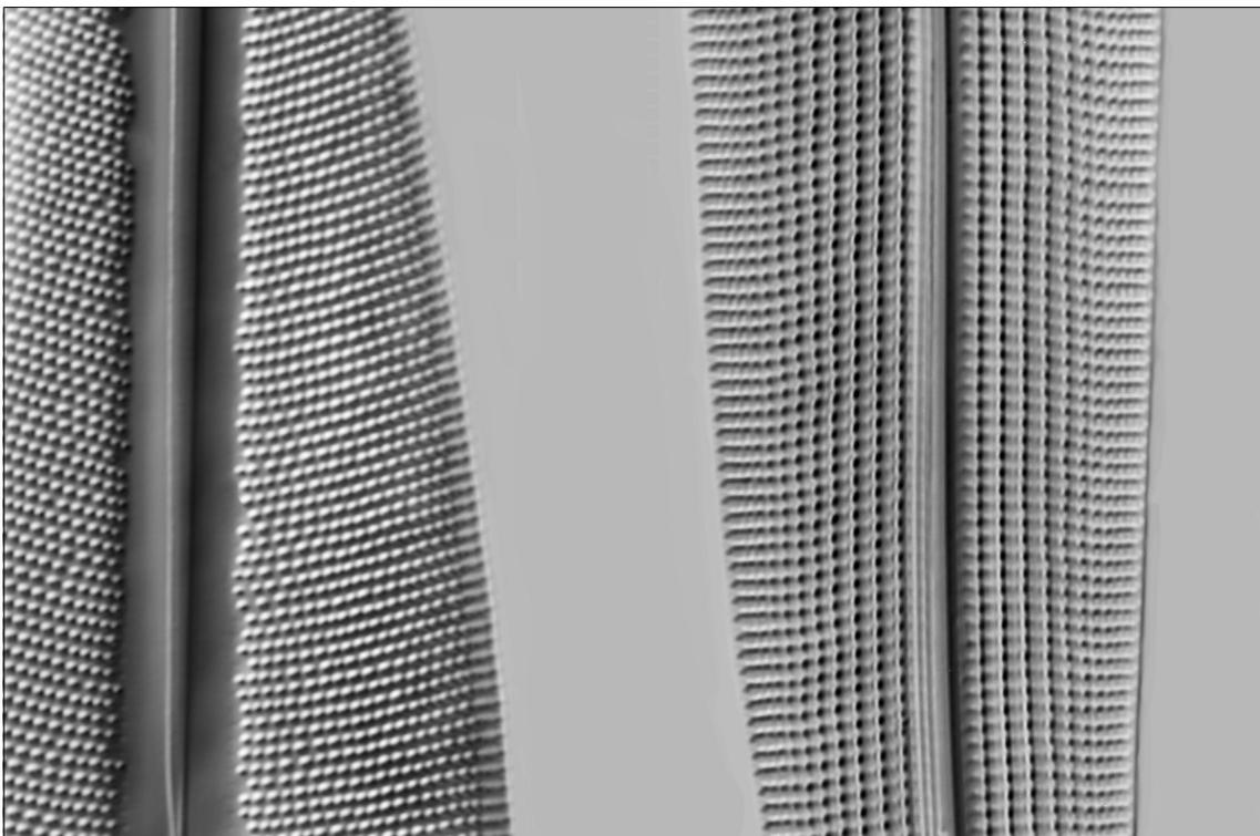
*Photo 6) The first two diatoms of the slide Diatom Test Slide Version 2.0 . Here they are perfectly resolved in oblique illumination with the Carl Zeiss Jena 40x / 0.95 lens with correction ring, mounted on the LwdE microscope.*
