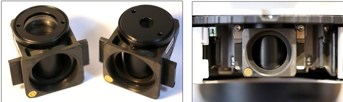
*Photo 2) Left. Two of the Optovar P & C Modules for Zeiss Axio Imager.A2 and Zeiss Axio Scope.A1 used in the Diatom Lab: 1.25x and 2.5x.*
